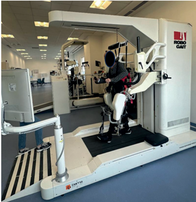
Figure 1. Robotic gait training system with body-weight support and lower limb exoskeleton components enabling controlled treadmill-based locomotor training. Source: Authors' own archive. The image has been anonymized to protect patient privacy
